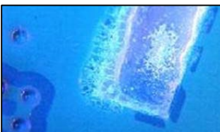
Flux residues causing coating uplift (photo courtesy of NPL)
